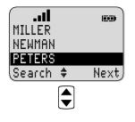
The three coloured keys (including the arrow key) below the display are known as softkeys. The functions associated with these keys are shown in the bottom line of the display. The function of the keys changes automatically, corresponding to the respective operating state of the handset.
